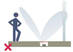
If the antenna angle is too small, the lobe will be reduced and reflected by the limits of the hole.
